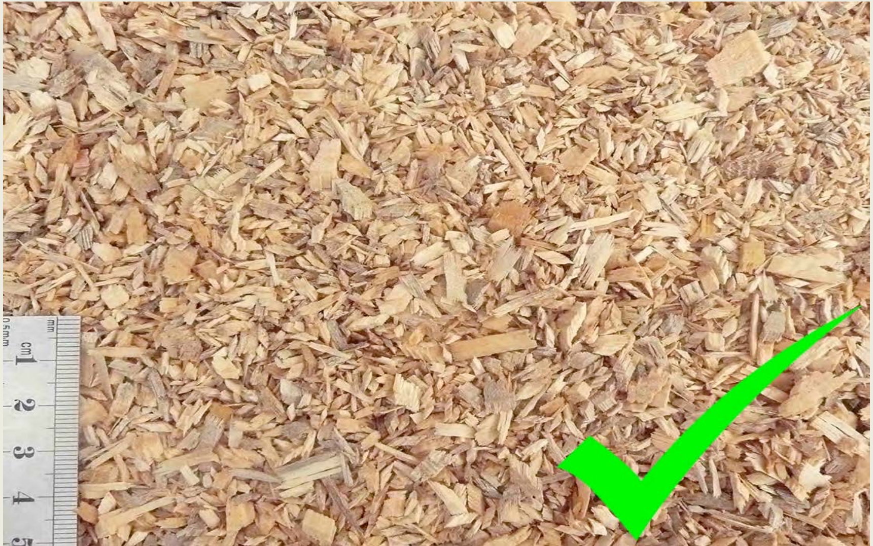
Figure D4 - uniform particle size, few sharps
