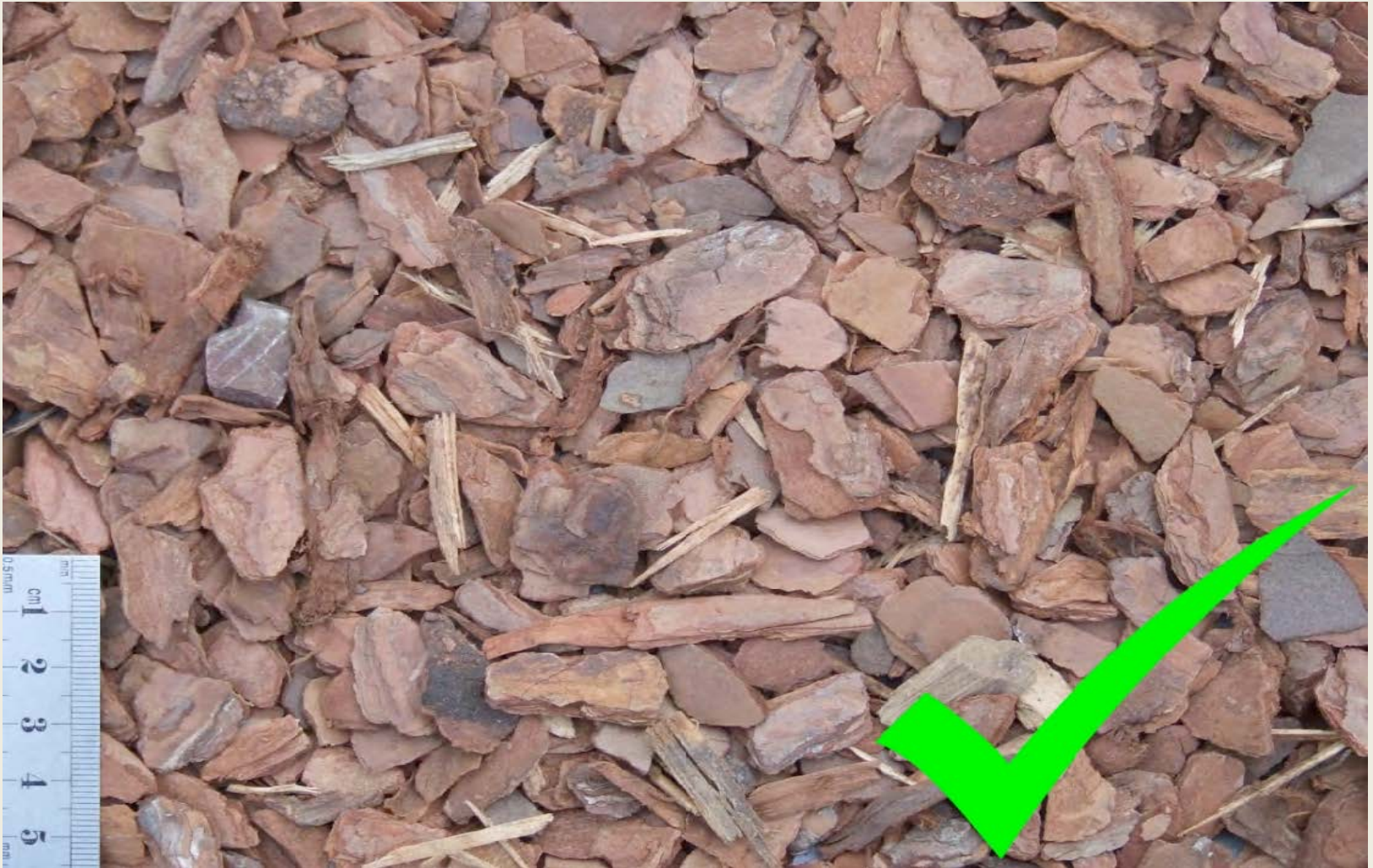
Figure D2 - uniform particle size, few sharps
