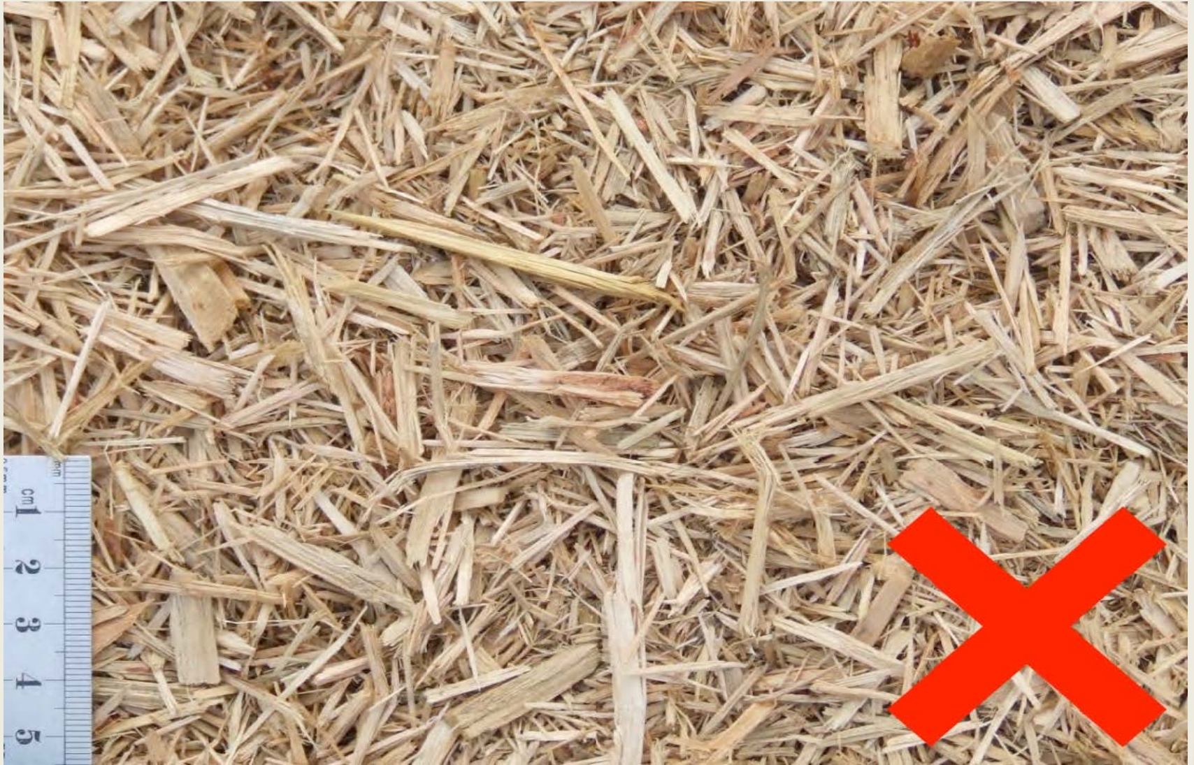
Figure D9 – many needle-like slender sharps with potential for splintering and puncture injuries
