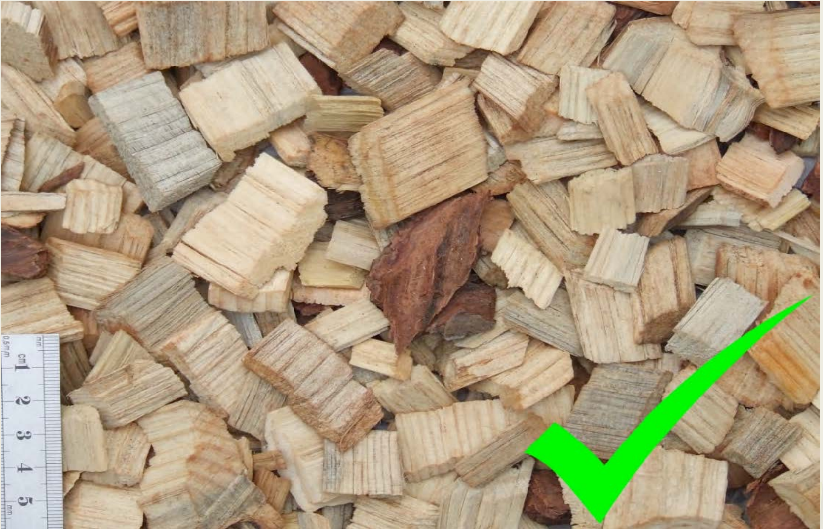
Figure D1 - uniform particle size, few sharps
