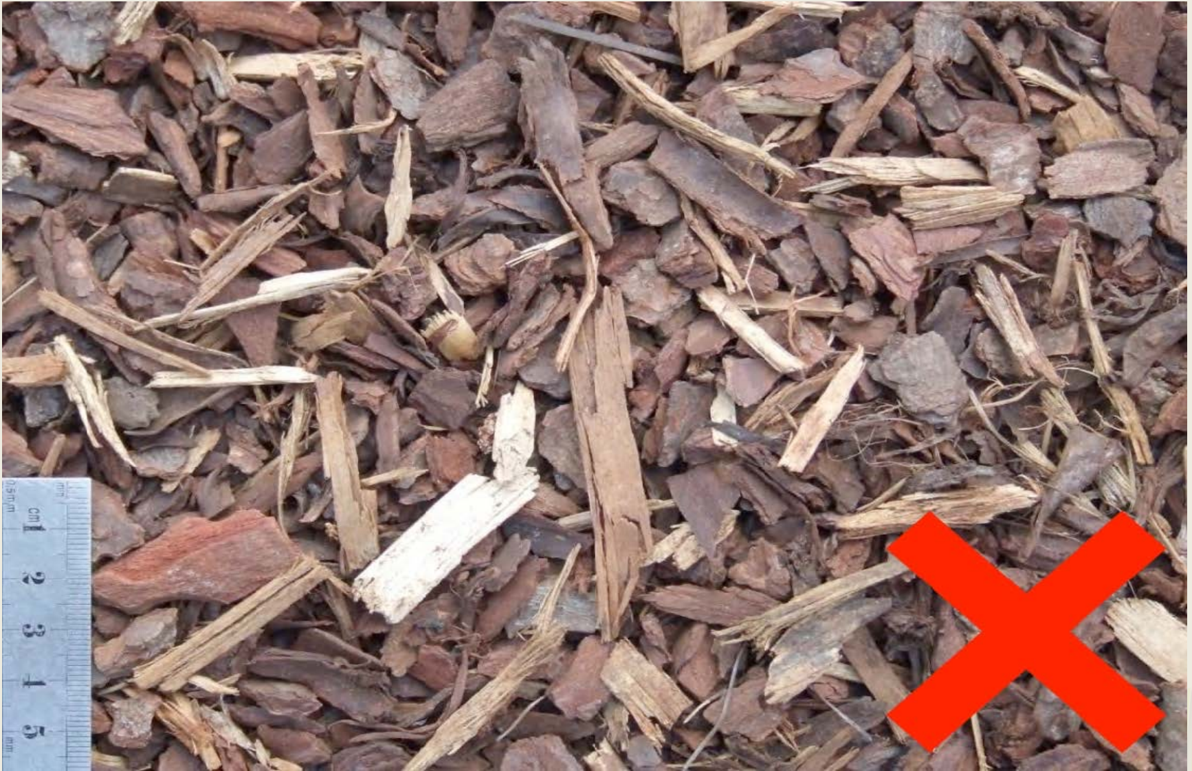
Figure D11 – large pencil-like pieces and sharp points with potential for splintering and puncture injuries
