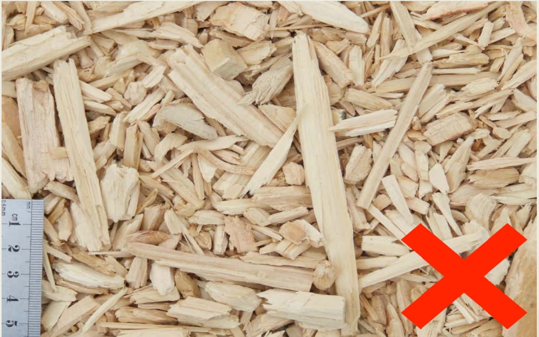
Figure D10 - large pencil-like pieces and sharp points with potential for splintering and puncture injuries
