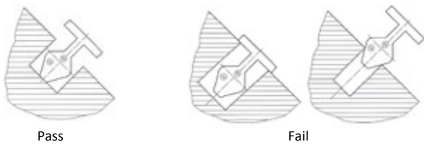
Figure 19 – Test method for partially bound and V-shaped openings
