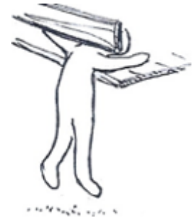
Figure 12 – Example of a bound opening that may cause head or neck entrapment
