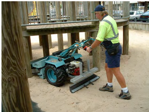
In-situ sieving using portable vibrating sieve
