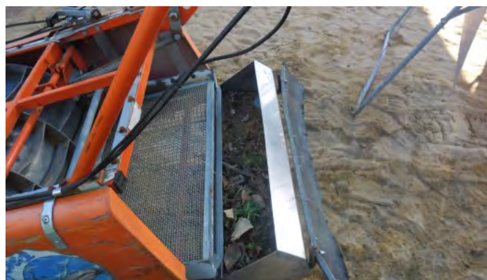
In-situ sieving using portable vibrating sieve
