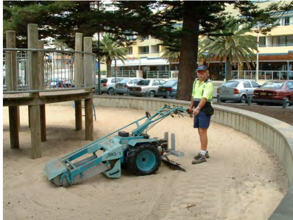
In-situ sieving using portable vibrating sieve
