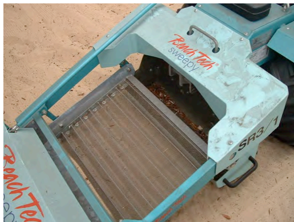
In-situ sieving using portable vibrating sieve
