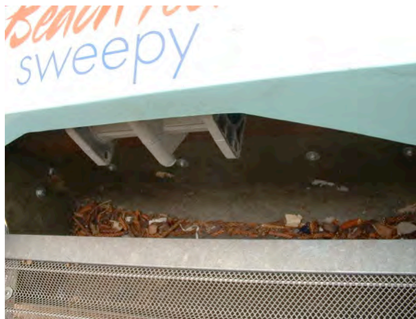
In-situ sieving using portable vibrating sieve
