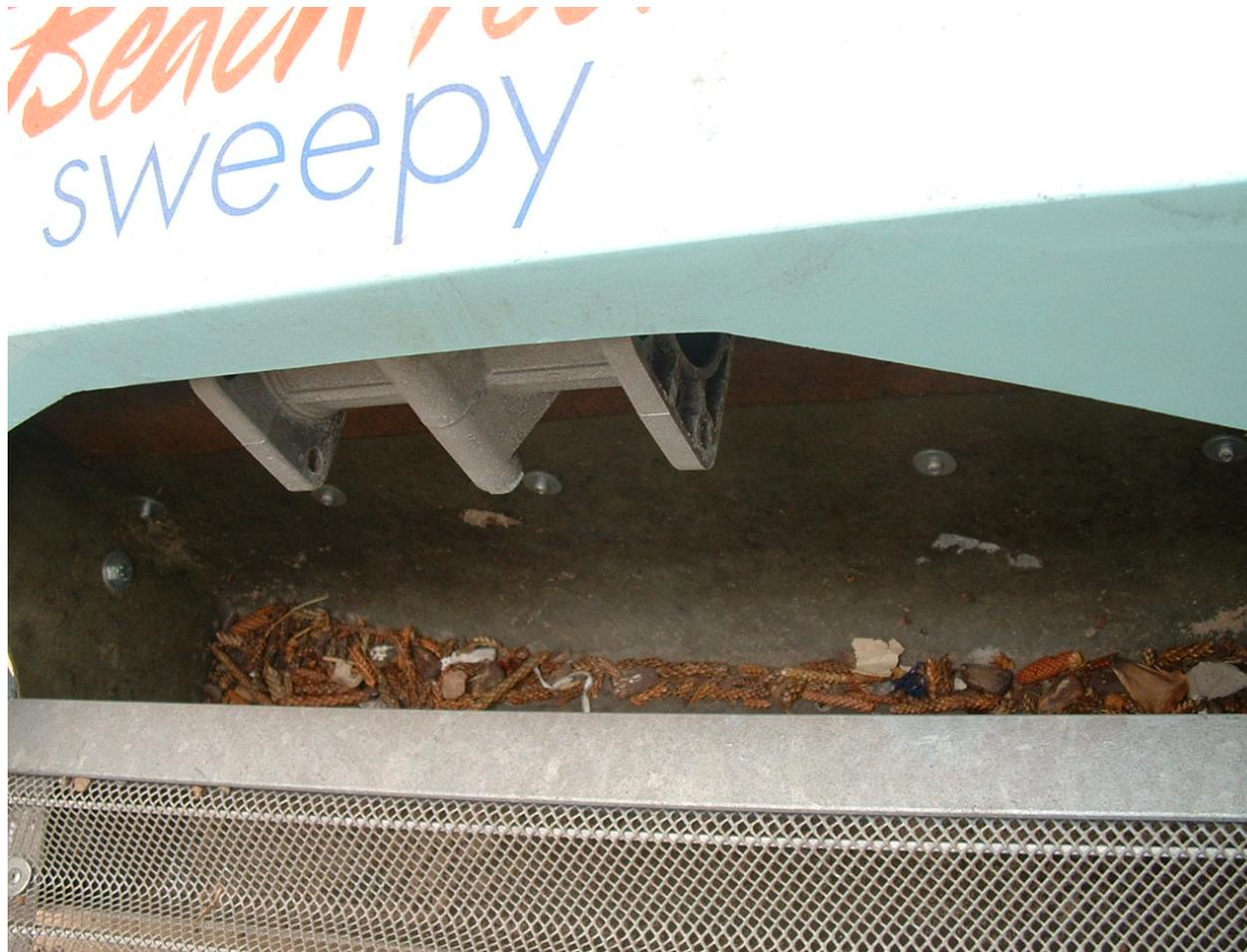
**In-situ sieving using portable vibrating sieve**
