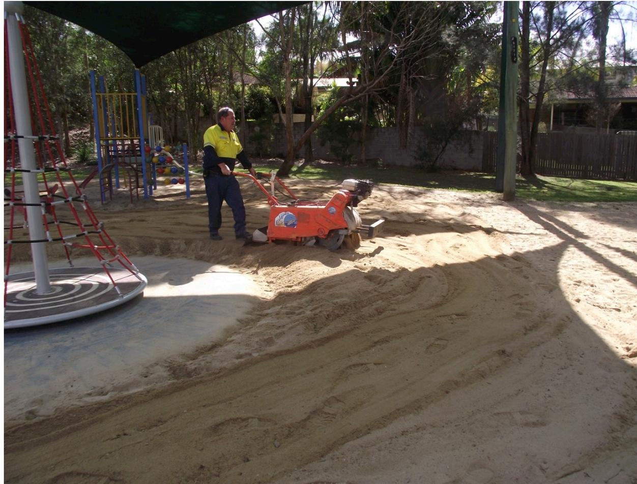
**In-situ sieving using portable vibrating sieve**
