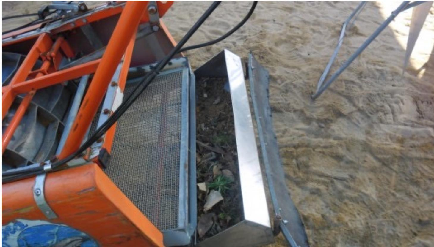
**In-situ sieving using portable vibrating sieve**
