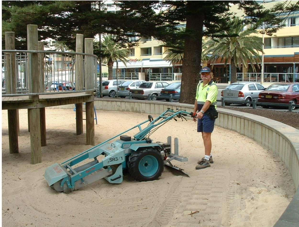
**In-situ sieving using portable vibrating sieve**
