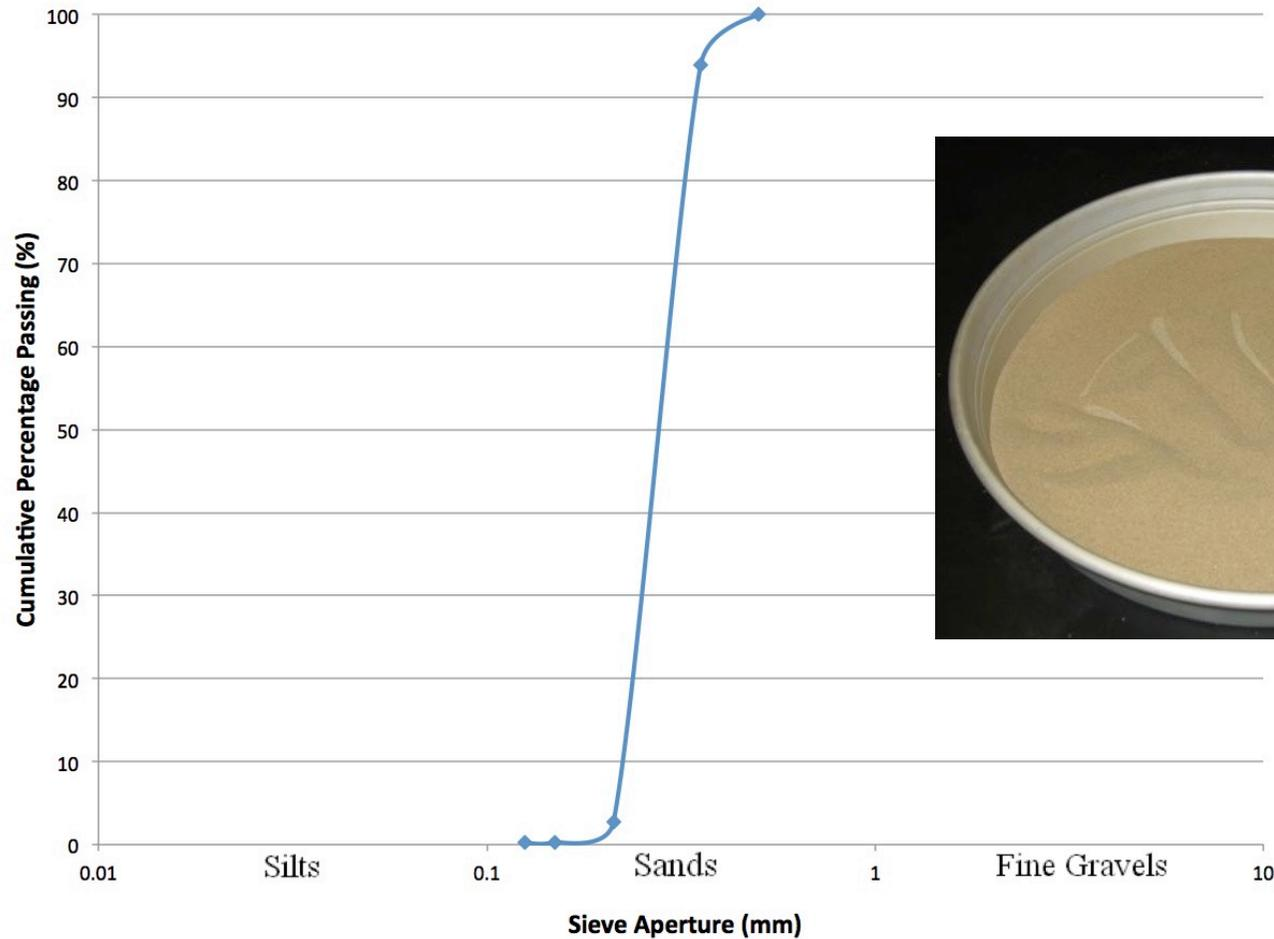
**Sand (fine): Sieve grading curve**
