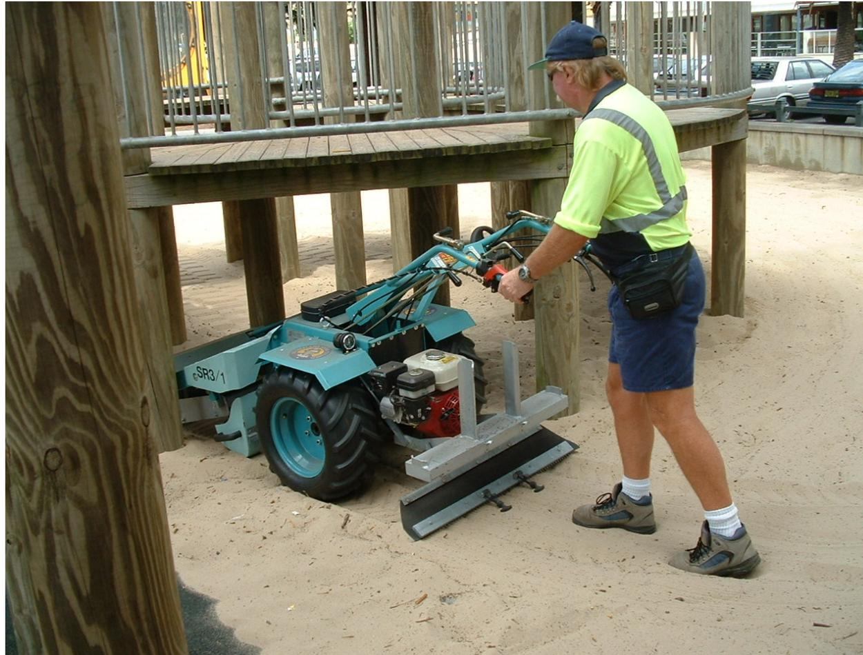
**In-situ sieving using portable vibrating sieve**
