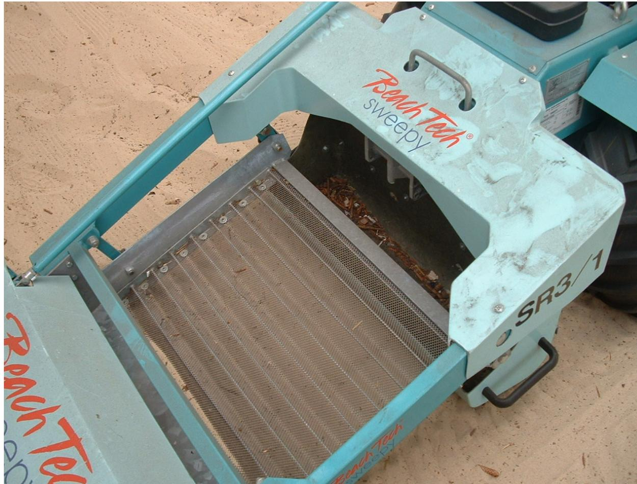
**In-situ sieving using portable vibrating sieve**
