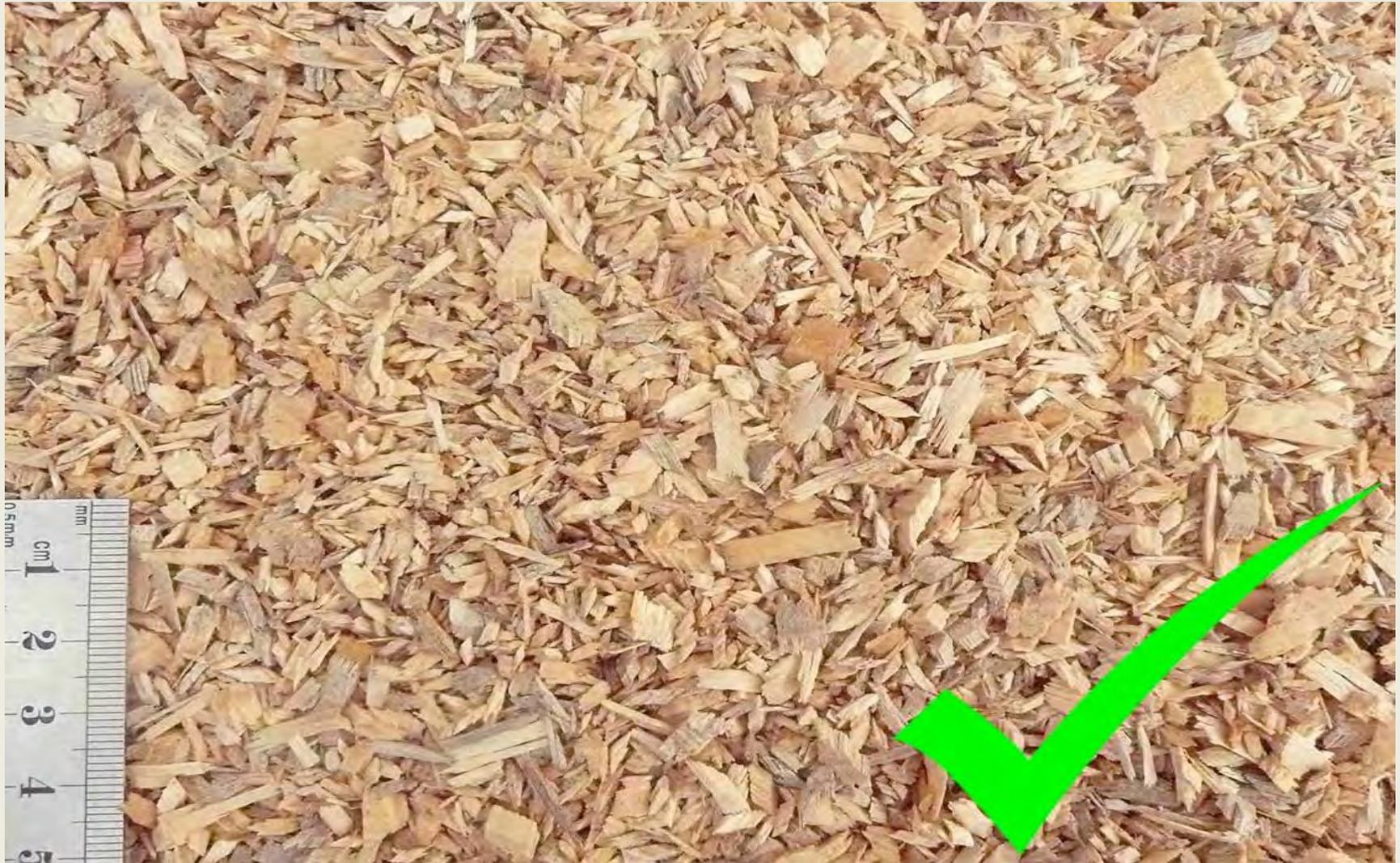
**Figure D4 - uniform particle size, few sharps**
