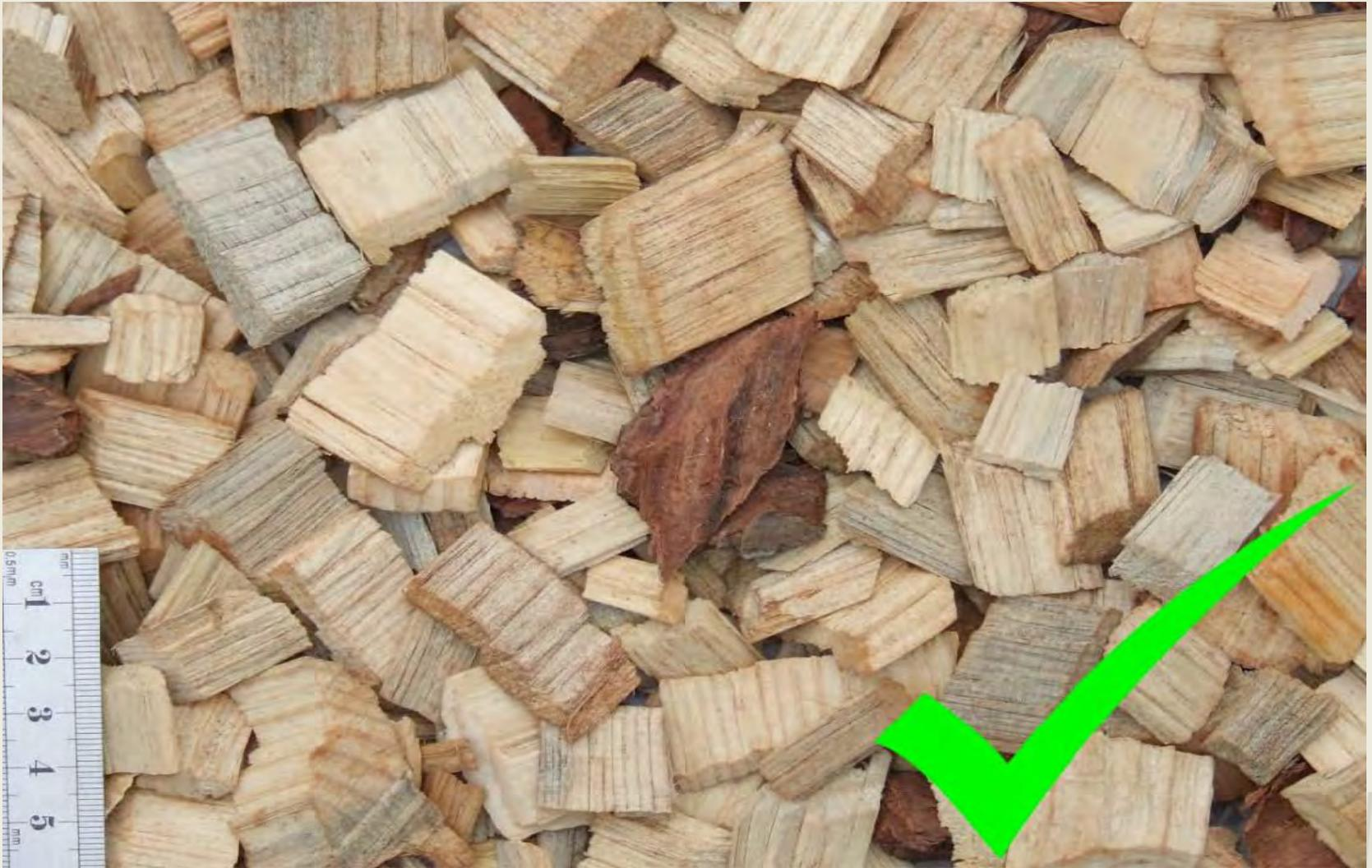
**Figure D1 - uniform particle size, few sharps**
