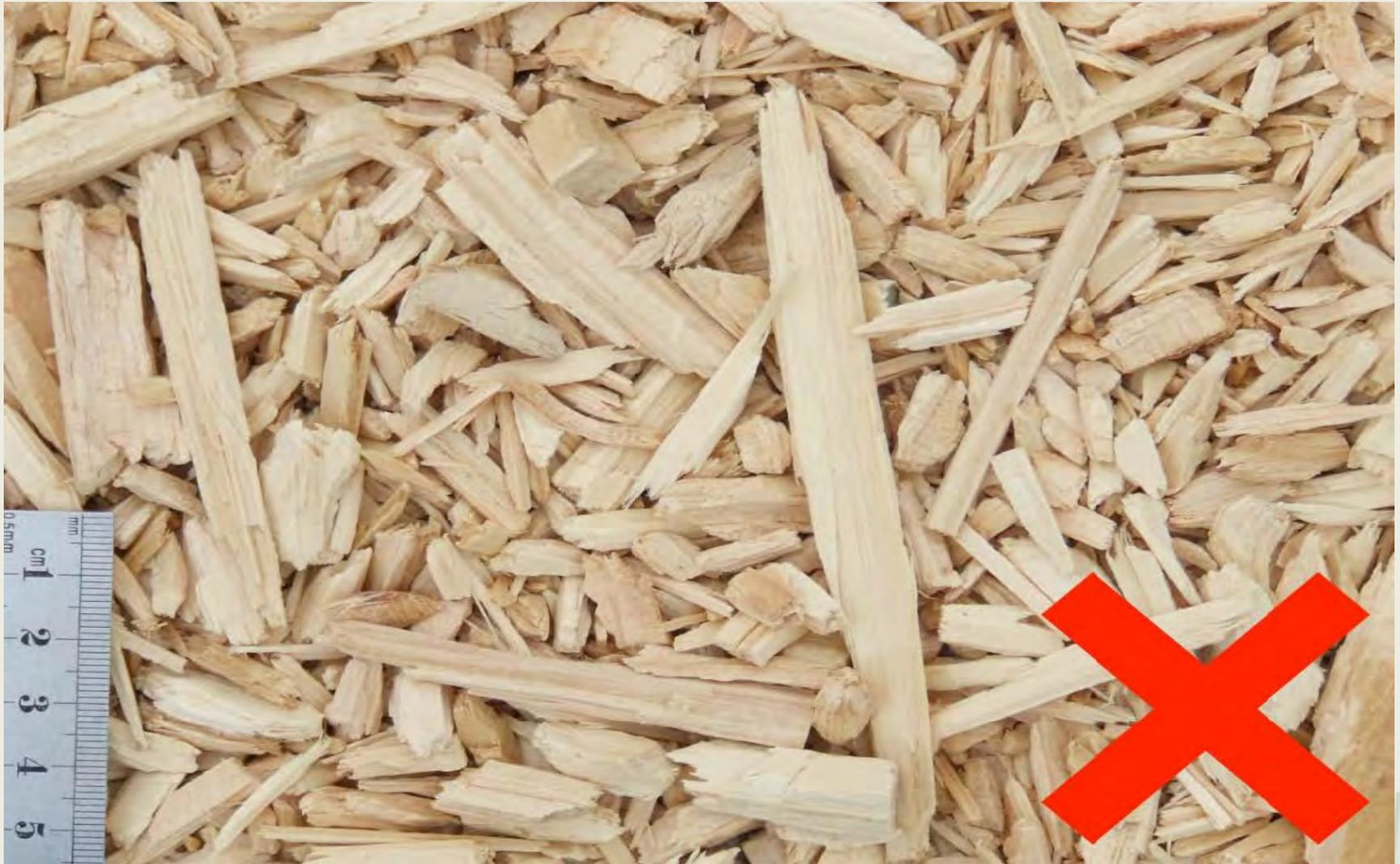
**Figure D10 - large pencil-like pieces and sharp points with potential for splintering and puncture injuries**
