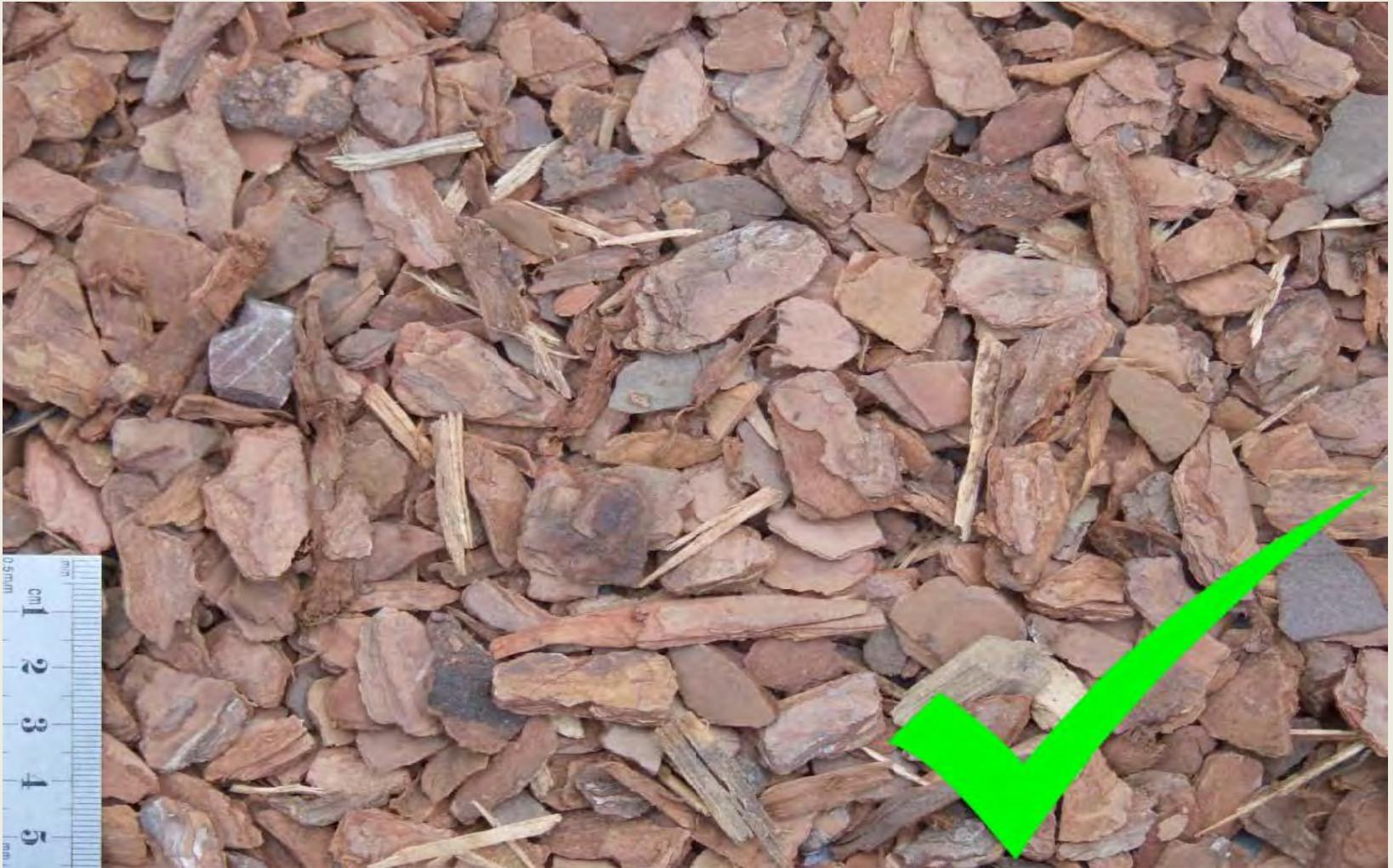
**Figure D2 - uniform particle size, few sharps**
