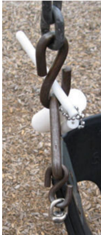
Fail 8.6mm probe fits 12mm probe doesn't
