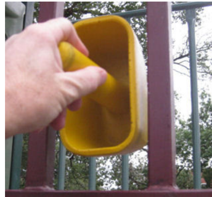
Barrier head entrapment (gap >89\text{mm} wide)
