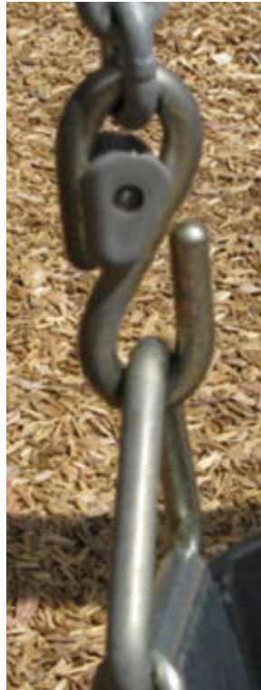
Fail & Pass! missing grommet
