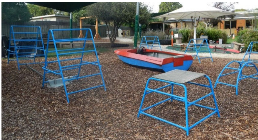
Well spaced equipment allowing falls to either side of the intended travel routes
