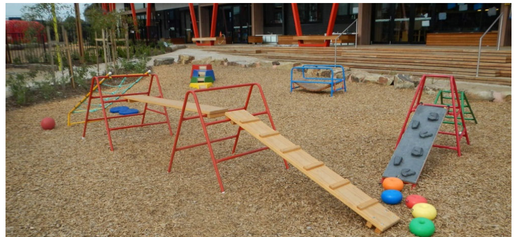
Well spaced equipment allowing falls to either side of the intended travel routes
