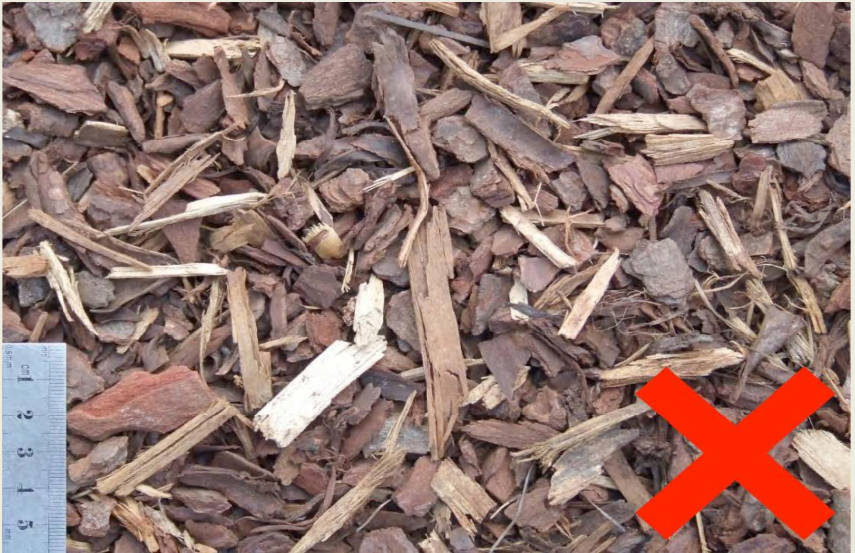
Figure D11 – large pencil-like pieces and sharp points with potential for splintering and puncture injuries
